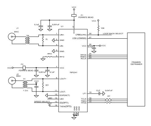
Note 6: Pin names in ( ) denote pin names from 78P7200. Pin numbers refer to 28 PLCC package. Default settings used to simulate 78P7200.
